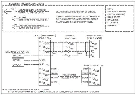
TS-3X-KT with LMV3, RWF10 load controller (LC), and RWF55 for water level controller (WL)
