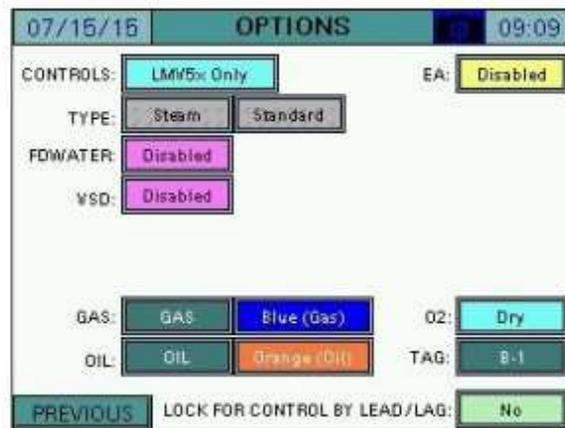
Once enabled, the **FEEDWATER** option on the main menu will be available, which allows access to the feedwater detail screen.
