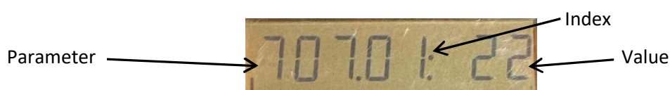
Figure 6-1: LMV3 Fault History Example with Indexes
