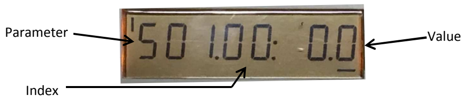
Figure 3-1: LMV3 Parameter Example with Indexes
