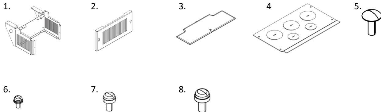
**Figure 15: Pieces Supplied with the DRN1-C1-5 NEMA 1 Kit**
