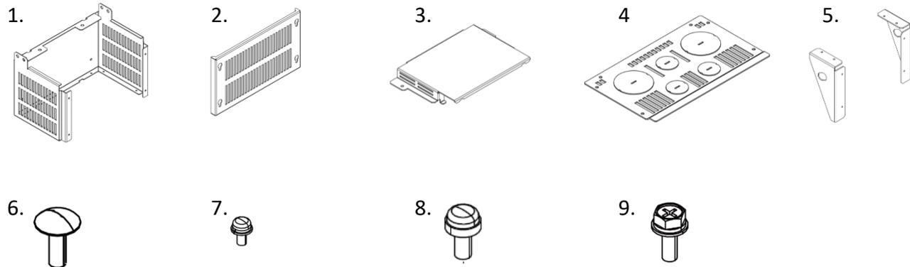
**Figure 21: Pieces Supplied with the DRN1-C1-6 NEMA 1 Kit**
