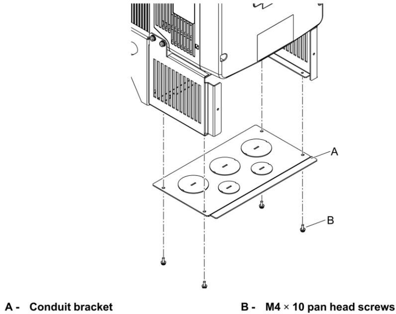
**Figure 19: Install the Conduit Bracket (DRN1-C1-5)**
