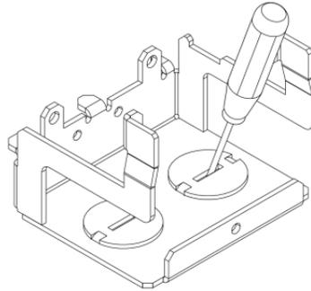
**Figure 10: Removing Knock-Out Holes (Procedure B DRN1-Bx-x)**
