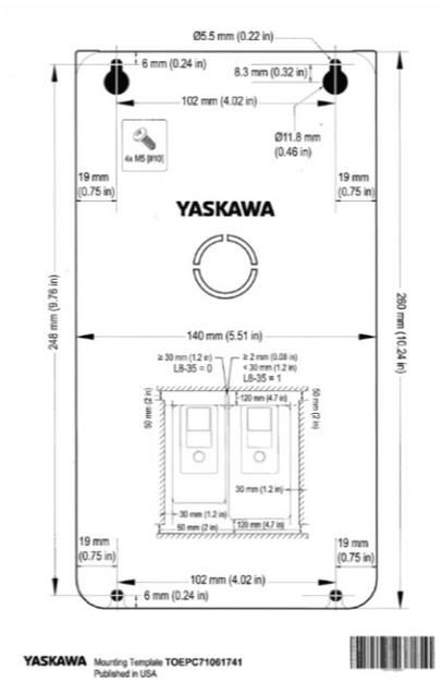
Figure 45: Example of a Template for Mounting
