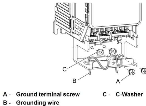
**Figure 13: Ground Wiring and Screws (Procedure B DRN1-Bx-x)**
