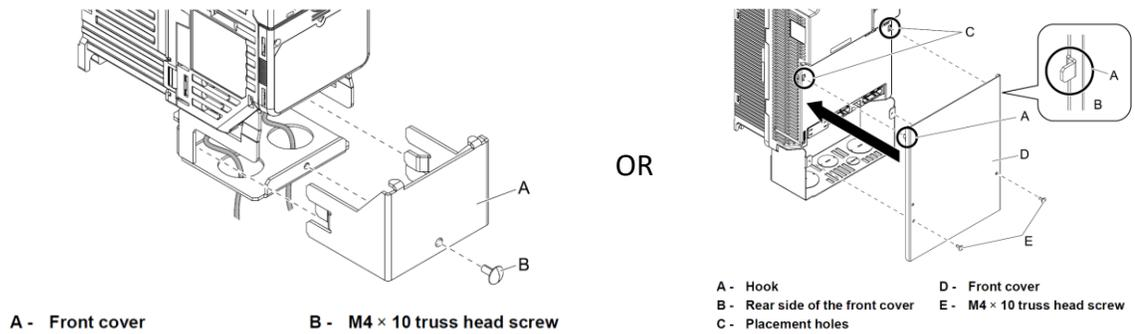
**Figure 14: Installing the Front Cover (Procedure B DRN1-Bx-x)**
