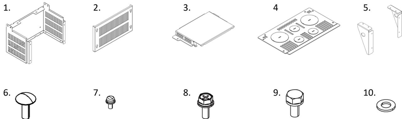
**Figure 29: Pieces Supplied with the DRN1-C1-7/8 NEMA 1 Kit**
