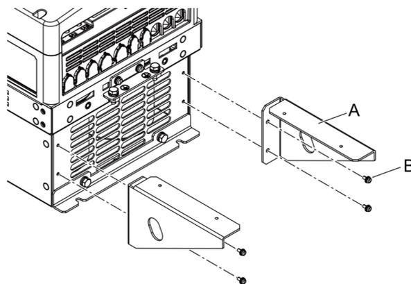
**A - Stay brackets****B - M4 × 8 pan head screws****Figure 32: Installing the Conduit Bracket (DRN1-C1-7/8)**
