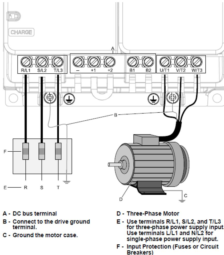
**Figure 51: Example Main Circuit and Motor Connections**
