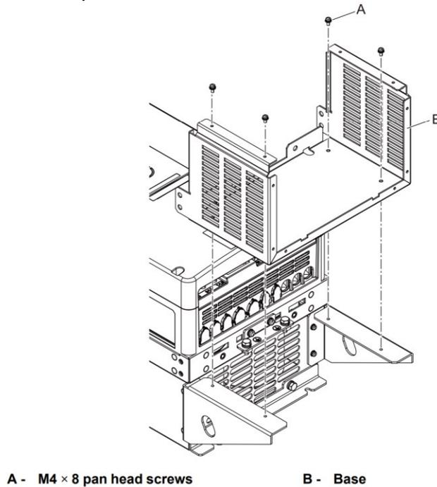
**Figure 25: Install the Base to the Stay Brackets (DRN1-C1-6)**
