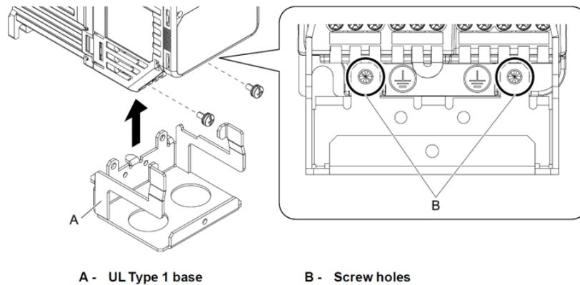
**Figure 12: Installing the Base (Procedure B DRN1-Bx-x)**
