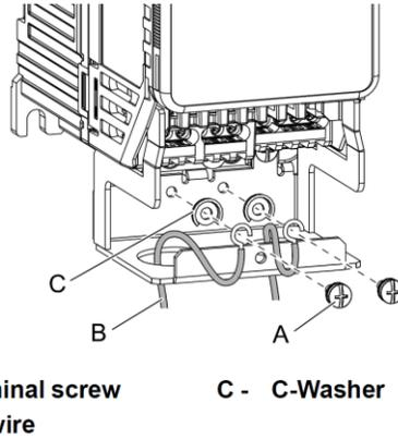
**Figure 6: Ground Wiring and Screws (Procedure A DRN1-Bx-x)**
