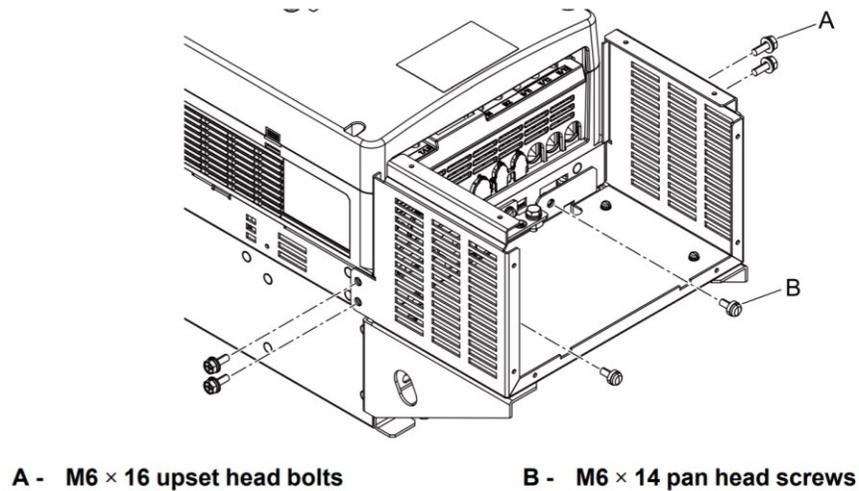
**Figure 26: Securing Base (DRN1-C1-6)**
