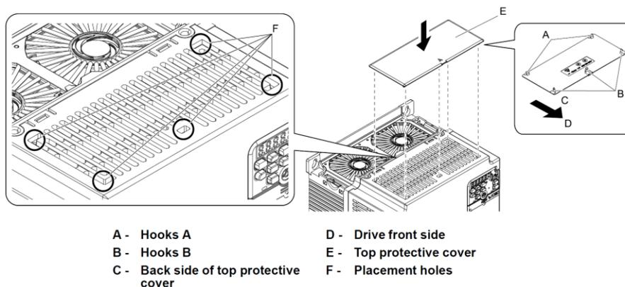
**Figure 9: Installing the Top Cover (Procedure B DRN1-Bx-x)**
