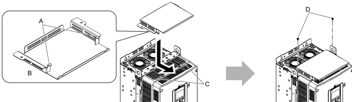
**A - Hooks****B - Underside of top protective cover****C - Placement holes****D - M4 × 8 pan head screws****Figure 31: Installing the Top Cover (DRN1-C1-7/8)**
