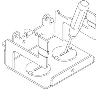
**Figure 3: Removing Knock-Out Holes (Procedure A DRN1-Bx-x)**
