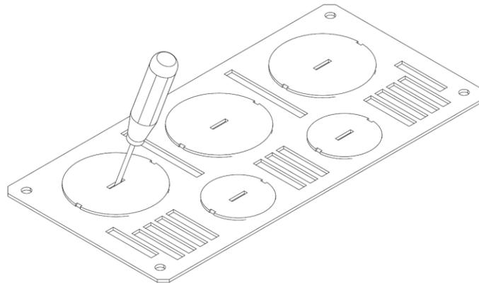
**Figure 16: Removing Knock-Out Holes (DRN1-C1-5)**
