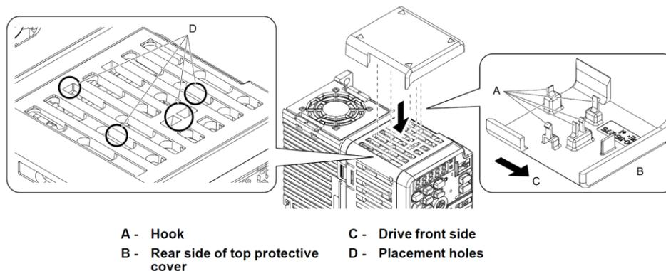
**Figure 2: Installing the Top Cover (Procedure A DRN1-Bx-x)**
