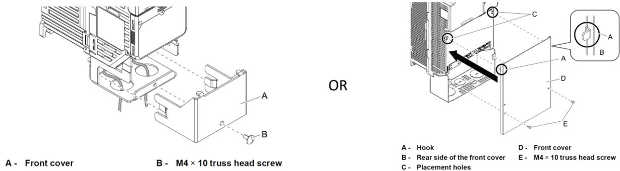
**Figure 7: Installing the Front Cover (Procedure A DRN1-Bx-x)**
