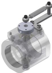
A manual kit with fine adjustment can be added to any VRG... butterfly valve for use as a flow restrictor. The kit allows for precision position adjustment. Locking nuts maintain the precise position at all rated flow pressures. To order AGA92.1 premounted on a VRG... butterfly valve, add a “-921” to the end of the VRG... valve part number. For example, the part number to order AGA92.1 premounted to a VRG10.050U valve is VRG10.050U-921.
