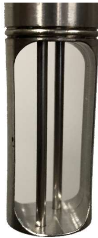
Figure 15: Clean Undamaged Probe
