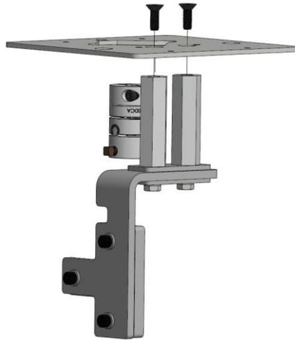
**Figure 5: Attach Actuator Bracket**
