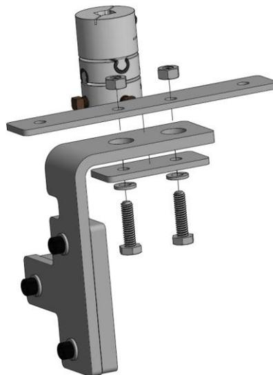
**Figure 4: Attaching Bracket Spacers**
