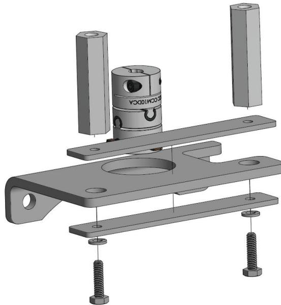
**Figure 5: Standoff Installation**
