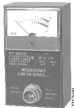
**KF8832** unit for measuring the detector current
