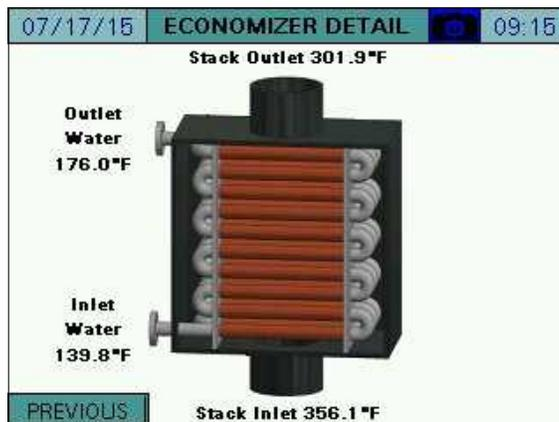
**Stack Inlet** – The stack temperature as it enters the economizer.
