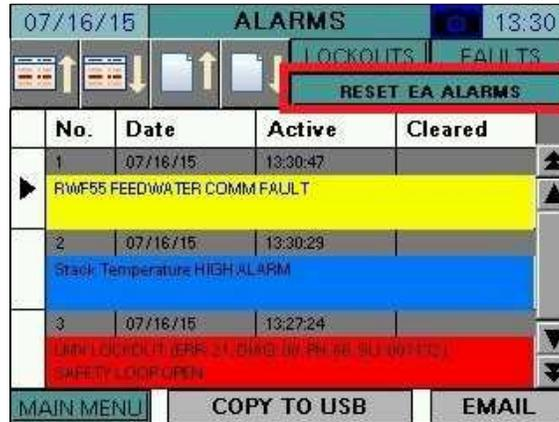
Press **COPY TO USB** to save the complete lockout or error history to a file (.csv). If email is configured, press **EMAIL** to send an email with the lockout or error history file attached. Note that a USB drive must be inserted to send email since the attached file is first stored on the USB drive.
