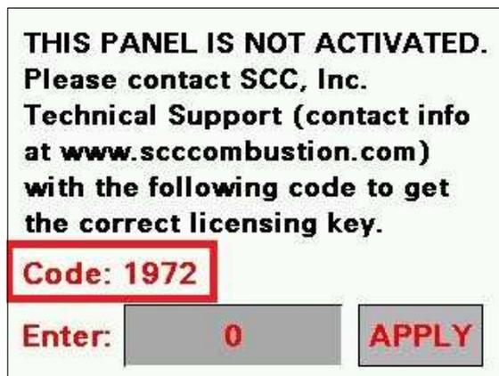
If the Expanded Annunciator is not activated, the activation screen will automatically appear when attempting to navigate to any Expanded Annunciator screen.
