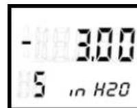
Press **Mode** again until parameter 6 is displayed. This is the maximum scaling. Enter a number that matches what was entered during the draft sensor setup using the **Up** and **Down** buttons. This should be a positive value.
