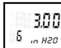
Press **Mode** repeatedly until parameter 14 is displayed. This is the display units. Choose "in H2O" using the **Up** and **Down** buttons. Close the access cover and the normal display screen will automatically return after 30 seconds.
