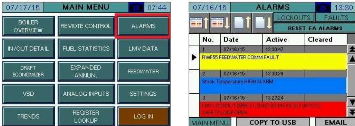
The ALARMS screen lists current alarms as well as older alarms. The color of the alarm indicates the category of the alarm:
