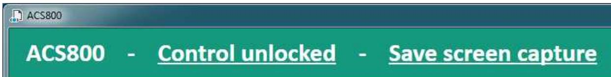
A screen capture of the current screen can be saved in the native resolution by clicking **Save screen capture**. The file format of the screen capture is png.
