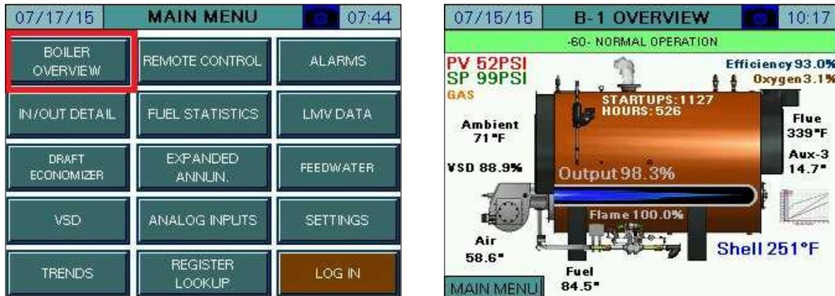
Only the parameters that are optioned and active are shown. Any others are hidden from the display for clarity. Touching the area displaying the O<sub>2</sub> trim data will display additional data. The following parameters may be shown on the overview screen:
