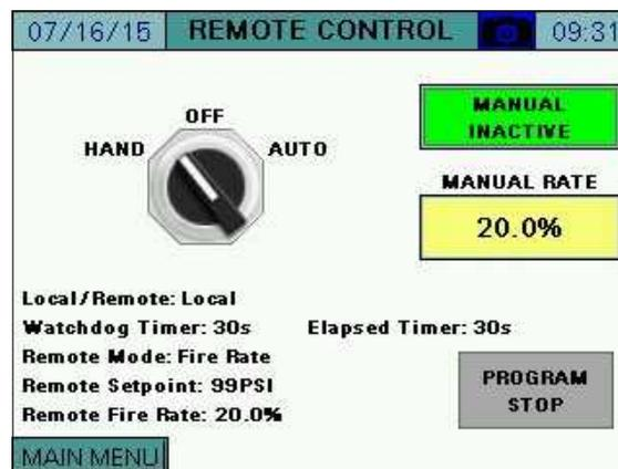
**HAND-OFF-AUTO** – Sets the mode of the boiler to manually on, manually off, or automatic. See **Table 2** for additional detail.
