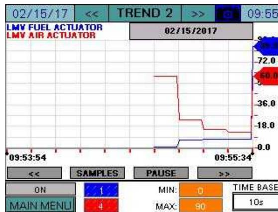
The USB drive must be inserted to use the trend option. Data will be stored for the previous 7 days.
