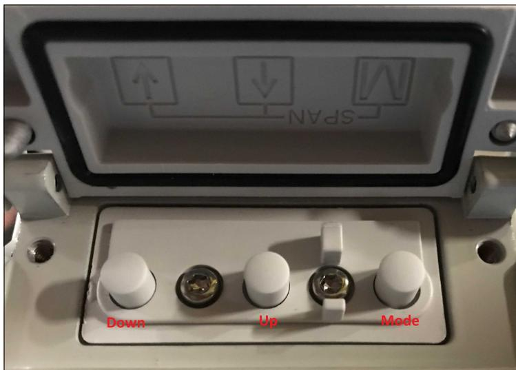
Press **Mode** repeatedly until parameter 5 is displayed. This is the minimum scaling. Enter a number that matches what was entered during the draft sensor setup using the **Up** and **Down** buttons, paying attention to the polarity as this should be a negative value.
