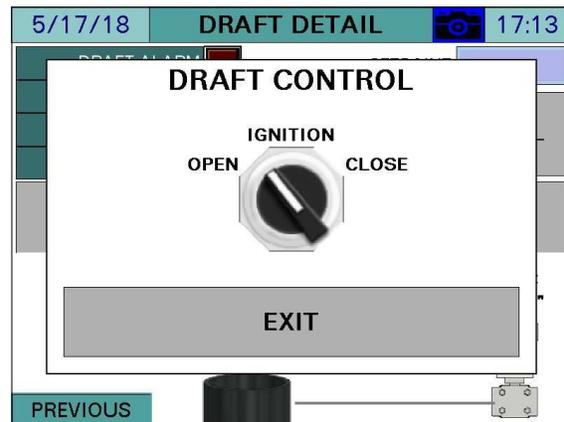
This allows the damper to be moved from the open to closed position easily.
