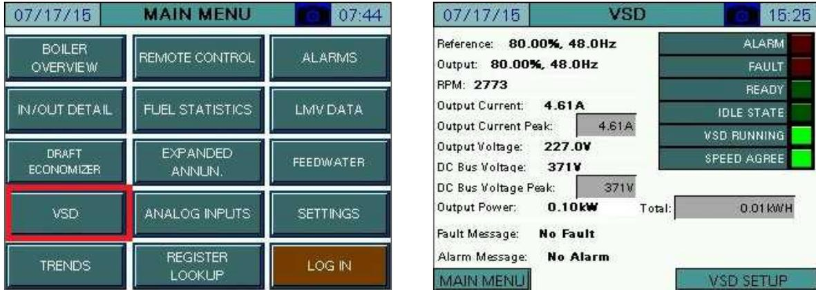
The peak output current and DC bus voltages are recorded during operation. To reset the peak readings, press the values for > 1s (hold down, TECH required).
