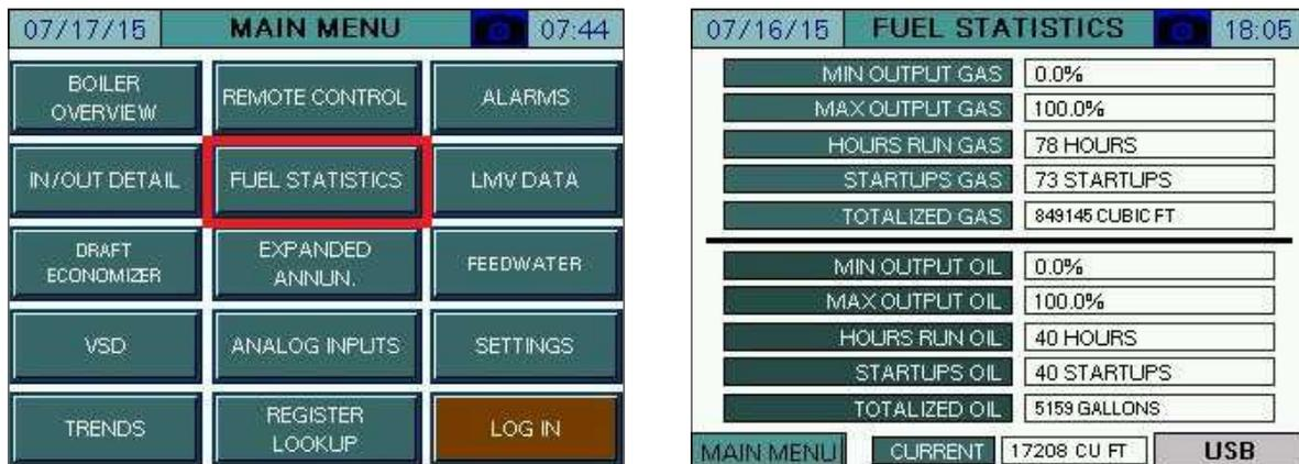
**MIN OUTPUT GAS/OIL** – Displays the minimum allowable load output programmed in the LMV controller.
