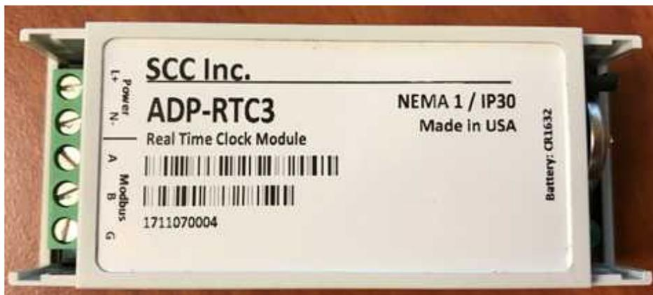
Install the ADP-RTC3 using DIN rail or the supplied foot mounts. The ADP-RTC3 can be powered with 24VAC or 24VDC. Connect to Modbus RS-485 as part of the chain of devices. Locating the ADP-RTC3 beside the OCI412.10 or OCI413.20 would allow sharing the same power and Modbus wiring.
