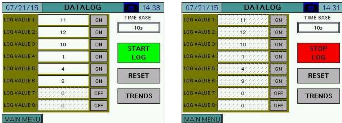
**LOG VALUES** – Sets the Modbus register index to log (TECH required).
