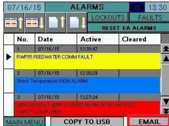
**NOTE:** If a boiler circulating pump is optioned with the Expanded Annunciator, an alarm is generated when feedback is not received within 20 seconds of the pump being commanded on. If this alarm appears, it must be reset using the **RESET EA ALARMS** button. The alarm will also automatically clear if pump feedback is received while an alarm is present.
