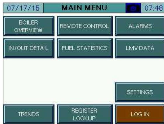
From here, different screens can be accessed depending on the access level. There are three access levels available:
