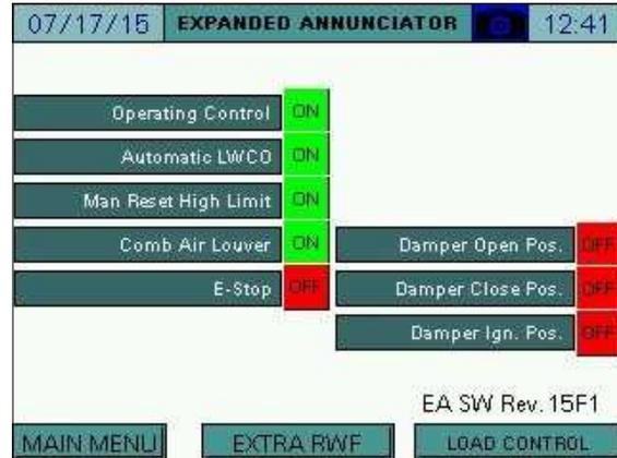
If extra RWF55 controls are optioned, press **EXTRA RWF** to access that screen. Press **EXP. ANNUN.** to return to the EXPANDED ANNUNCIATOR screen.
