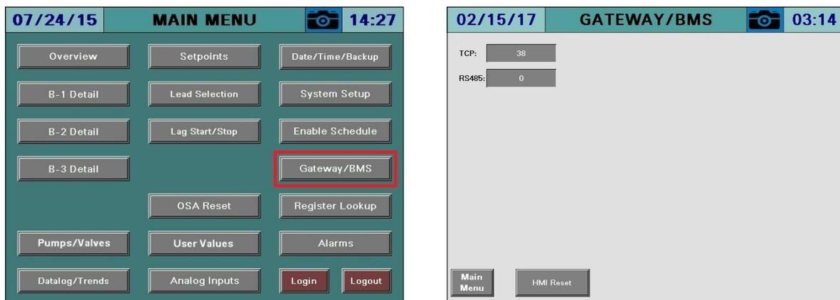
Incoming communication statistics for each of the interfaces are shown. Holding down the value for > 1s (hold down) will reset that interface's statistics to zero.
