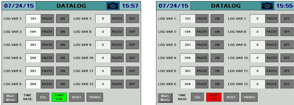
**LOG VALUES** – Sets the Modbus register index to log (TECH required).
