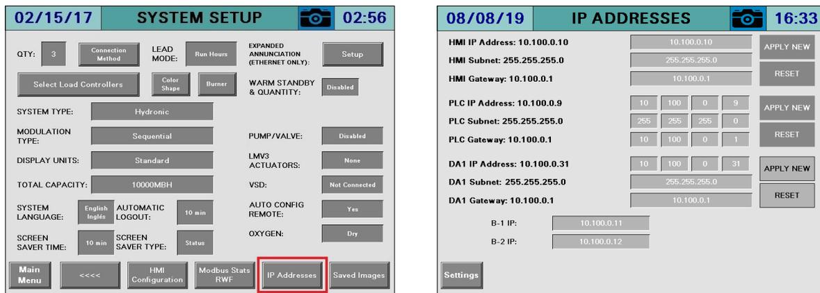
To toggle between the HMI (ETHERNET1) and BMS (ETHERNET2) IP addresses, touch the area marked **1** for > 1s (hold down). To toggle between the connected DA1 and DA2 IP addresses, touch the area marked **2** for > 1s.
