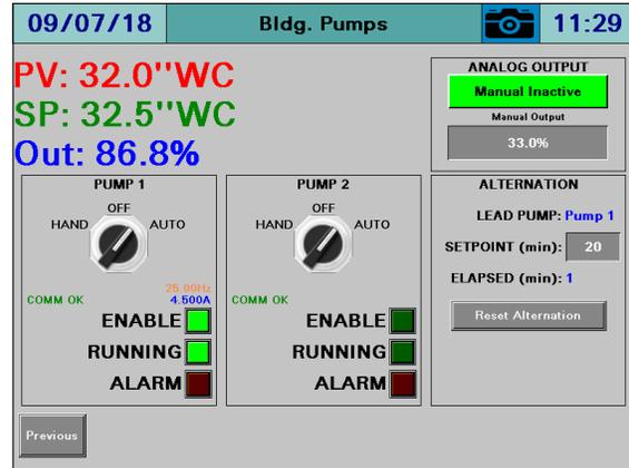
**PV:** Displays the loop process variable. If there are multiple process variables specified, the controlling process variable will also be shown.
