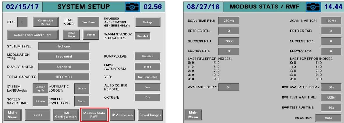
This allows adjustment to the Modbus master parameters for RTU and TCP as well as monitoring of the current communication statistics.
