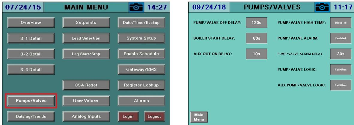
In a hydronic system, boiler circulating pumps or isolation valves can be cycled with the boiler. If there are four or fewer connected boilers, an auxiliary output with a separate on-delay timer is available.
