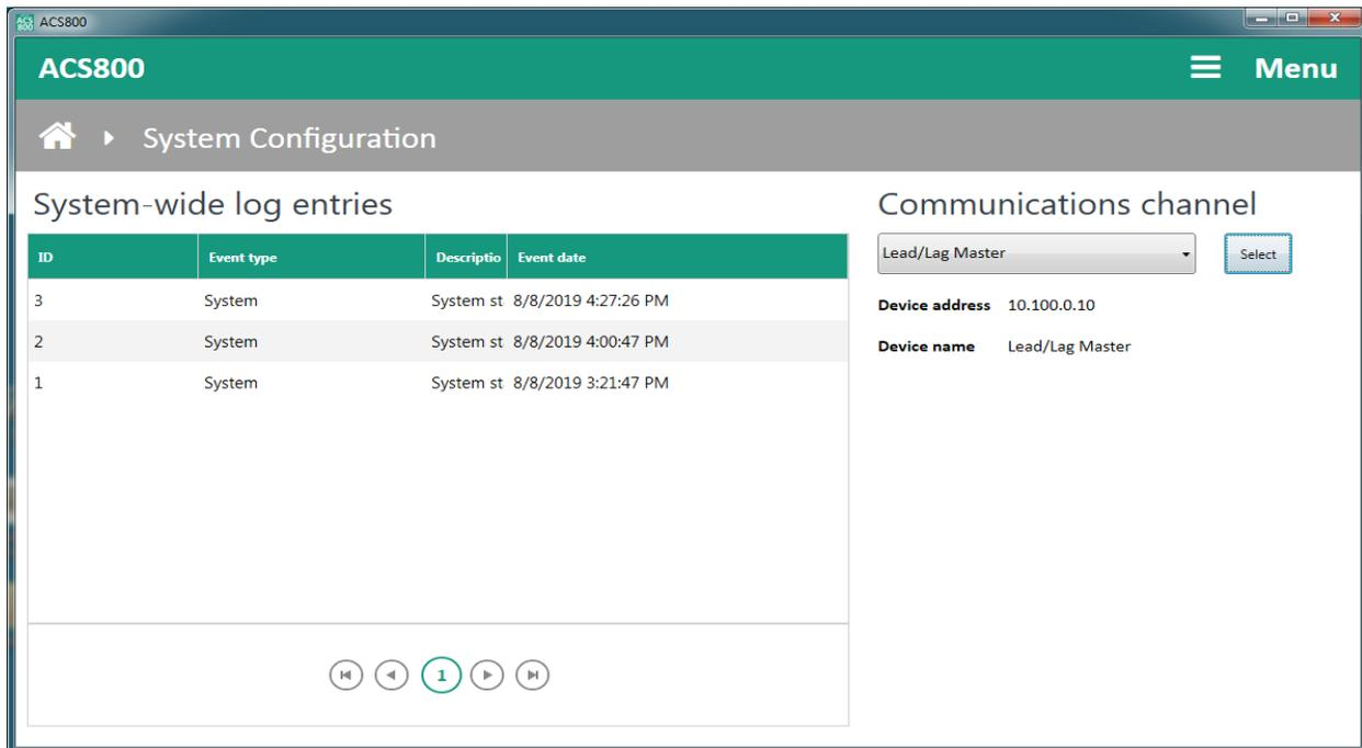
Choose the device to connect in the drop-down menu under the **Communications channel** tab. Choose **Lead/Lag Master** to connect that device if it uses the default IP address of 10.100.0.10. If the Lead/Lag Master uses a different IP address, choose **Other** from the menu and enter the IP address desired. Click **Update** to identify the remote device. Once the device is connected, click **Submit** to complete the connection.
