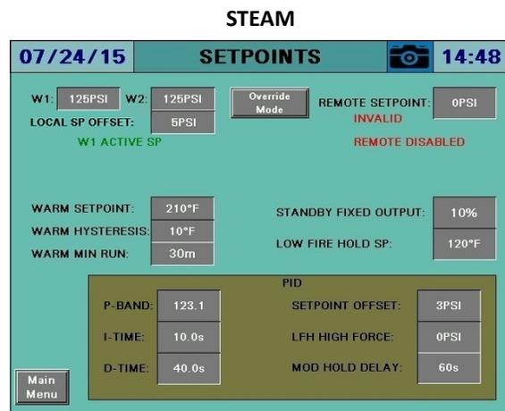
**Warning:** The connected LMV must be commissioned using accurate fuel flow metering. Failure to do so may result in poor performance since the required firing rate will not correspond to a linear burner output. It may not be possible to find suitable PID settings to control under this scenario since the feedback will not be representative.
