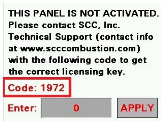
If the lead/lag controller is not activated, 'MASTER NOT ACTIVATED' will appear on the SYSTEM SETUP screen. Press **Master Activation** to enter the activation code.
