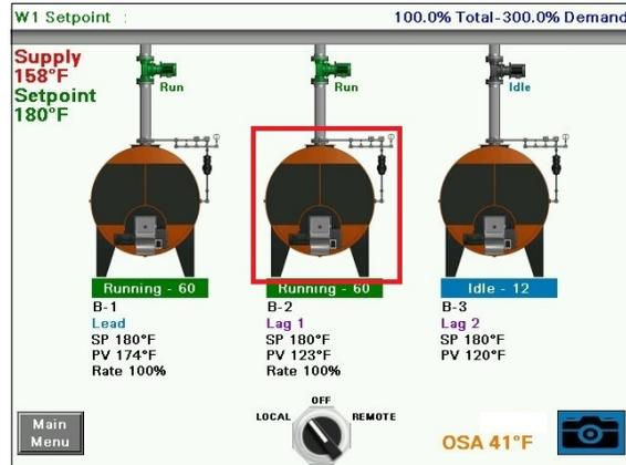
Touching the boiler information will display the boiler HAND-OFF-AUTO switch (see *Boiler Overview* → *Hand-Off-Auto* section for additional detail).
