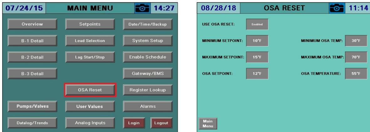
The setpoint can be generated based upon the outside air temperature. The outside air temperature sensor is polled once every five minutes to update the current setpoint (maximum 12 setpoint changes per hour). If the outside air temperature reading is invalid or the sensor becomes inoperative, the default setpoint will be used.
