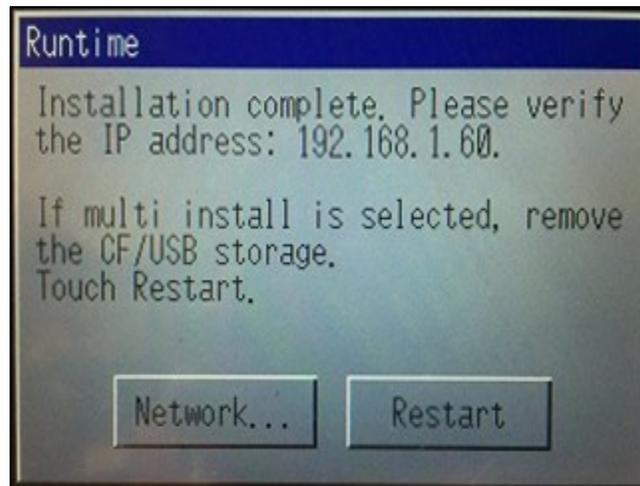
The device will then reboot with the new software and the process is complete. If an activation is necessary, contact SCC Inc. technical support with the activation code displayed and enter the key given to complete the activation process.
