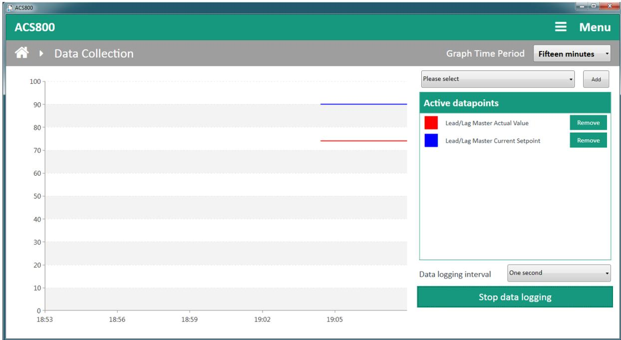
To stop the data logging, click **Stop data logging**. The data will be available for export until another data log is initiated. A data log will only continue logging if the ACS800 software is running and the log is active.
