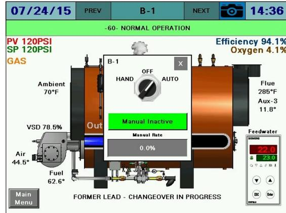
**HAND-OFF-AUTO** – Sets the mode of the boiler to manually on, manually off, or automatic. See **Table 4** for additional detail. The position will synchronize with the HAND-OFF-AUTO switch located on the touchscreen kit, if applicable.
