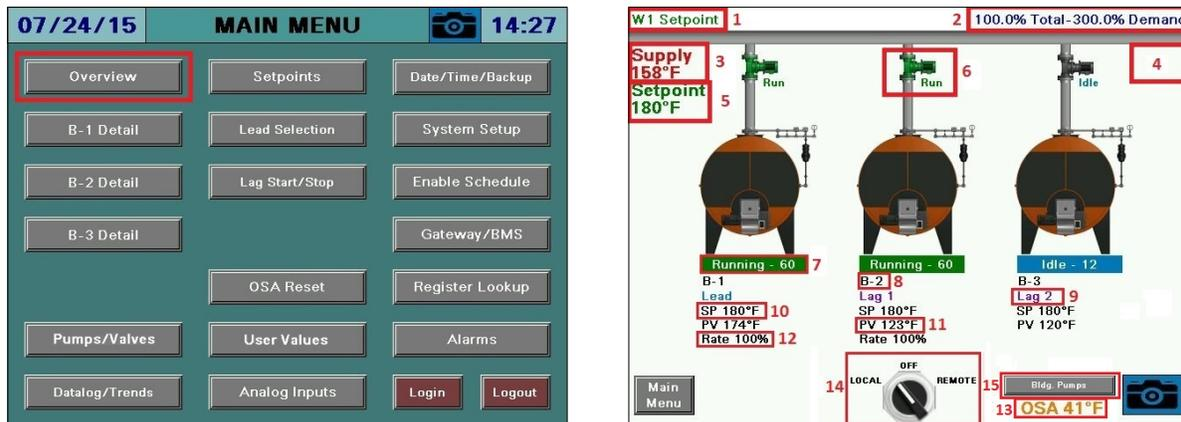
Only the parameters that are optioned and active are shown. Any others are hidden from the display for clarity. The following parameters may be shown on the overview screen (reference legend number for location on screen):
