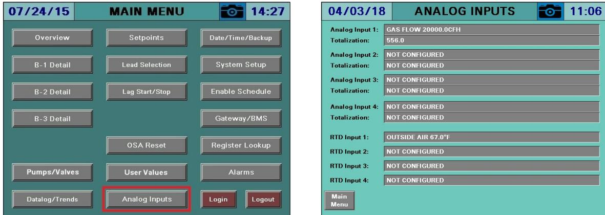
If totalization is enabled for any of the analog inputs, touching the totalized value > 1s (hold down) will reset the value to 0 (TECH required).
