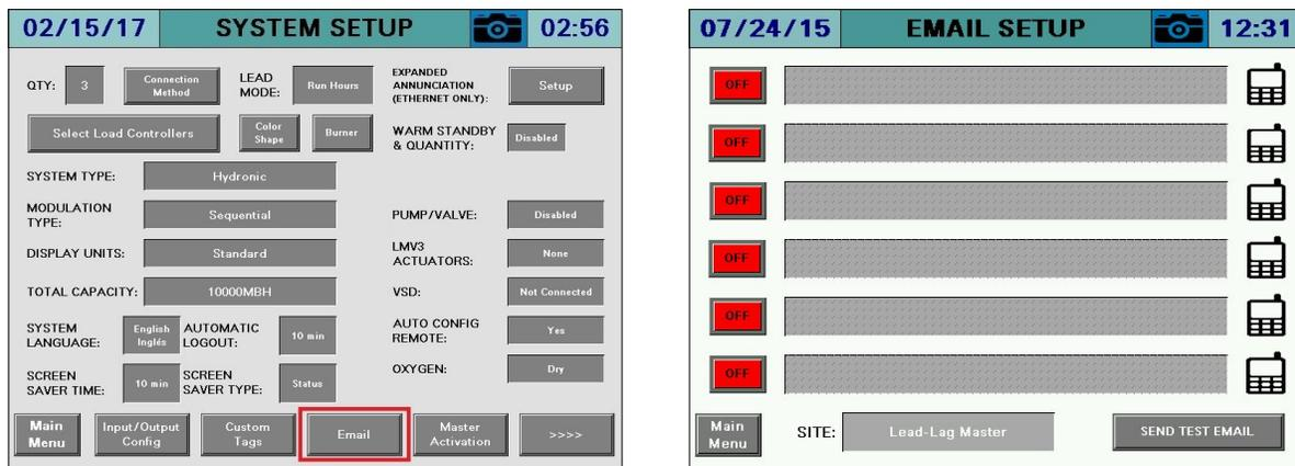
The touchscreen can be configured to send email to up to six addresses. This requires that the touchscreen is connected to a network with Internet access. Emails are sent automatically when alarms occur and may be sent manually to send screen captures and other data from the touchscreen. To configure an email address, press the **ON/OFF** button to the left of the address line, then enter the address.
