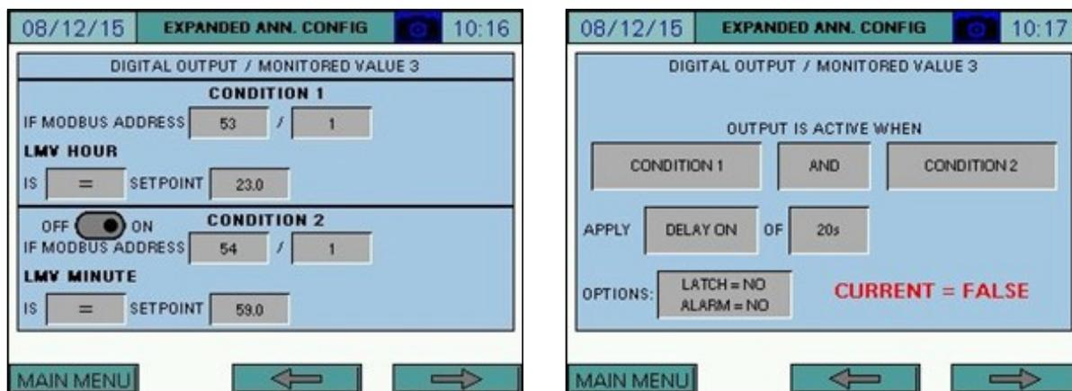
If desired, the action can be latched and/or create an alarm when true. Latching would require a manual reset via the ALARMS screen to clear the condition.
