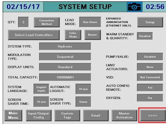
Press the >>>> then press the **HMI CONFIGURATION** button. Once the HMI CONFIGURATION screen is displayed, press the **OFFLINE** tab.
