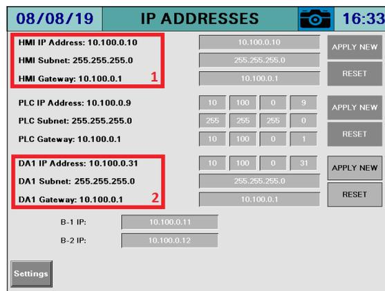
When changing the IP address for the HMI, BMS, PLC or either connected DA, touch **APPLY NEW** for > 1s (hold down) to apply the entered setting. Touch **RESET** for > 1s to return to the default IP address for that device. Changing the IP address for any touchscreen kit will take effect upon entry.
