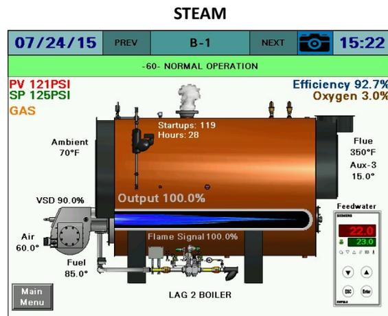
Use the **PREV** and **NEXT** buttons to navigate between boilers.
