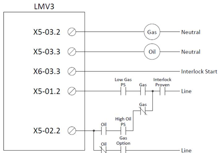
Set parameter 214 (Max Time Start Release) to a value long enough to ensure that the external device will prove open at every start. This parameter holds the LMV3... in phase 22 until terminal X5-01.2 or X5-02.2 has been proven.
