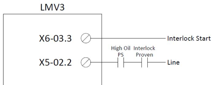
If the unit uses both fuels, wire relays to X5-03.2 (fuel 0 selected) and X5-03.3 (fuel 1 selected). These relays are necessary to prevent back feeding voltage and to bypass other gas options required to connect to X5-02.2 such as high gas pressure, POC or valve proving (shown as "Gas Option").
