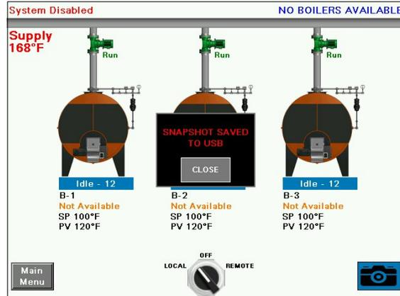
If there is no USB drive inserted or there is an error while trying to save the snapshot, a message will display saying 'SNAPSHOT SAVE ERROR'.
