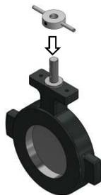
2. Line up set screw with the smaller notch in the valve shaft.
