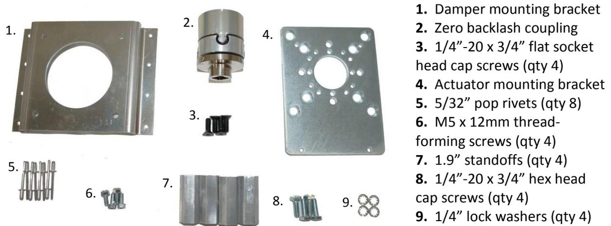
**Figure 1: Components Included in a Lucoma Air Damper Bracket Assembly**
