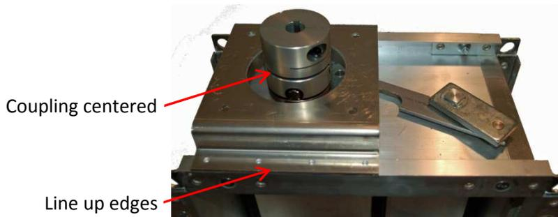
**Figure 7: Aligning Bracket with Coupling**
