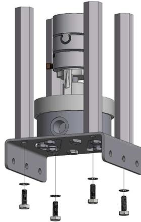
**Figure 6: Standoff Installation**
