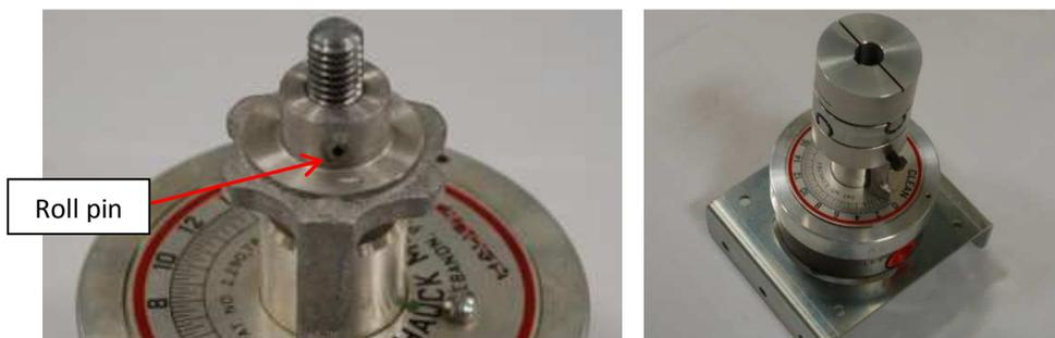
**Figure 5: Coupling Installation**
