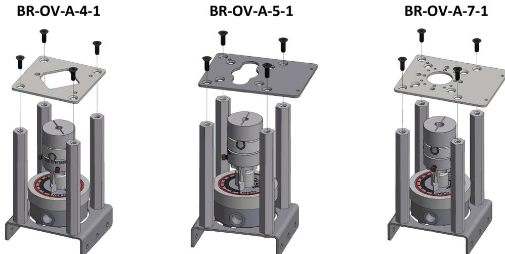
**Figure 7: Actuator Mounting Bracket Installation**
