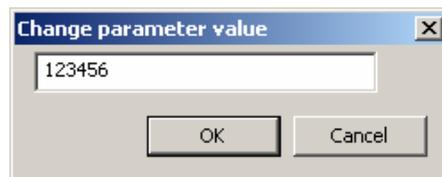
Here, a maximum of 8 digits for the burner's ID can be entered.
