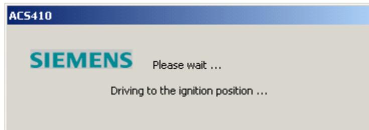
The burner control travels to the ignition position. To ensure the burner control stops at the ignition position, the ACS410 automatically sets a program stop.
