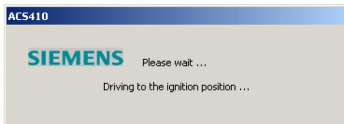
The burner control travels to the ignition position. To make certain it stops there, the ACS410 automatically sets a program stop.
