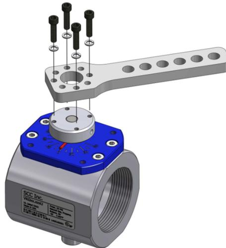
**Figure 3: Crank Arm Installation**
