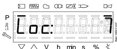
The display shows **Loc.**. The bar under the fault status message
