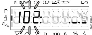
On the left, parameter **102:** is displayed flashing.
