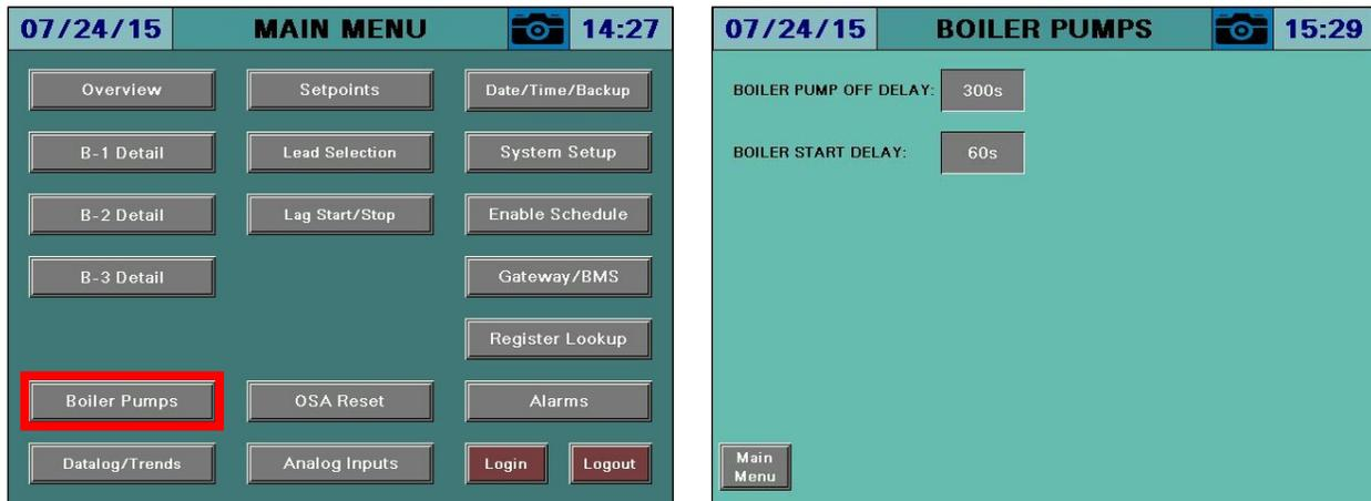
In a hydronic system, boiler circulating pumps or isolation valves can be cycled with the boiler.
