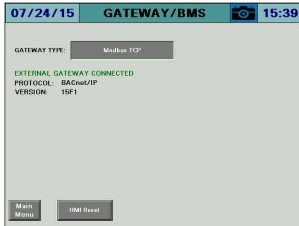
If a TS Series Protocol Converter is connected, 'EXTERNAL GATEWAY CONNECTED' will appear. The configured protocol and version is also displayed.
