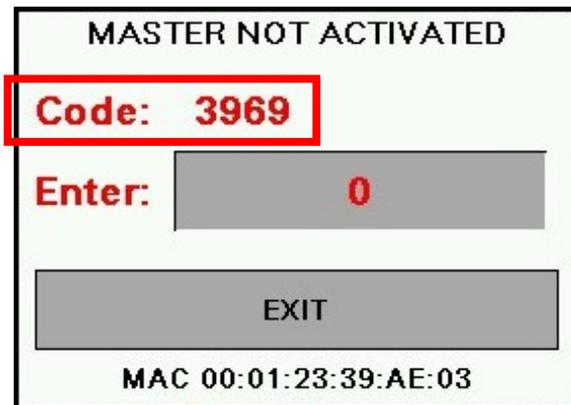
Contact SCC, Inc. technical support with the code listed and an activation key will be provided. Once it is entered, press **APPLY**.
