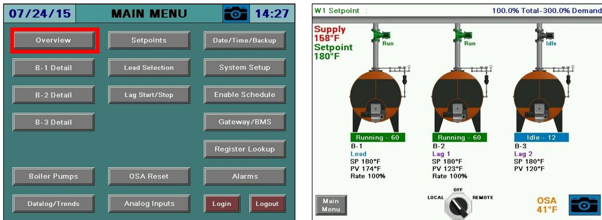
Only the parameters that are optioned and active are shown. Any others are hidden from the display for clarity. The following parameters may be shown on the overview screen:
