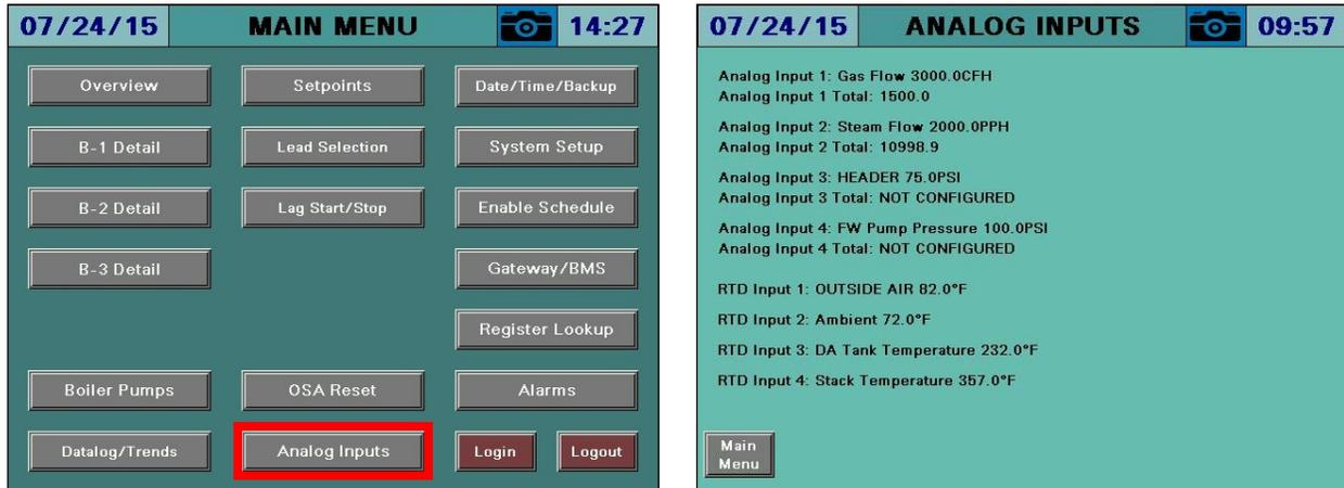
If totalization is enabled for any of the analog inputs, touching the totalized value > 1s will reset the value to 0 (TECH required).
