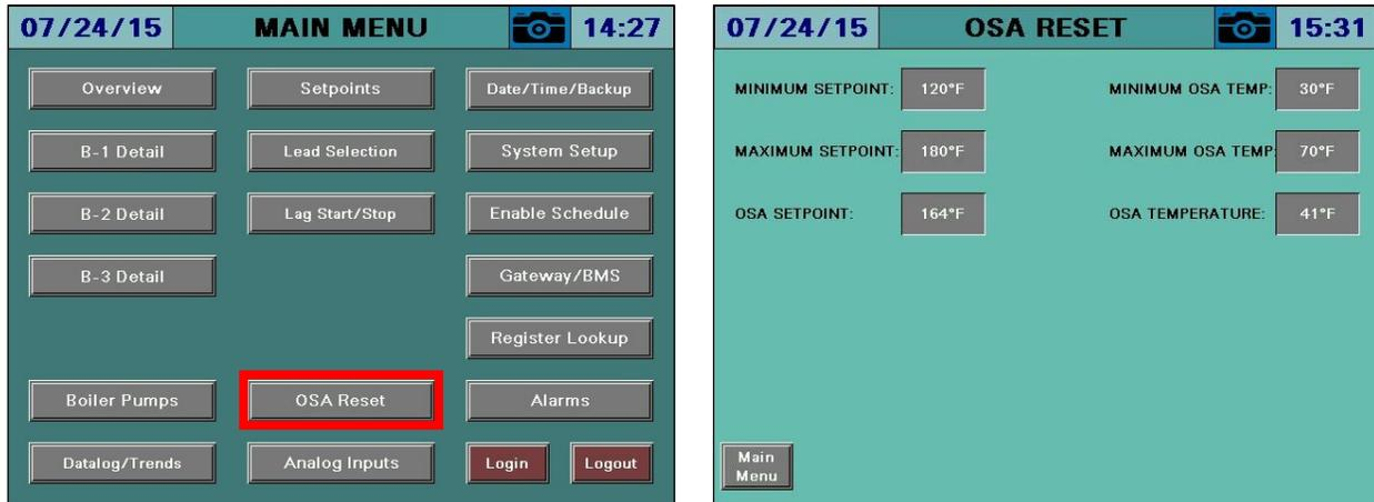
In a hydronic system, the setpoint can be generated based upon the outside air temperature. The outside air temperature sensor is polled once every five minutes to update the current setpoint (maximum 12 setpoint changes per hour). If the outside air temperature reading is invalid or the sensor becomes inoperative, the default setpoint will be used.
