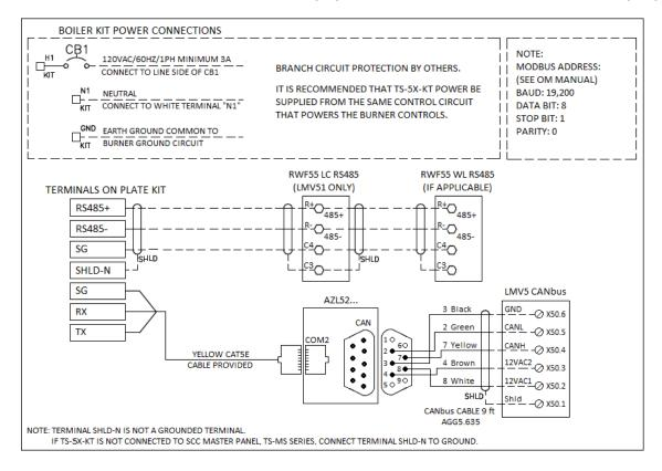
**Note:** For all RS-485 connections, use Belden Cable 3106A (multi-conductor cable with twisted pair, EIA Industrial RS-485 PLTC/COM) or equivalent.
