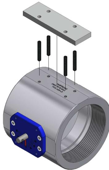
**Figure 2: Placing the Spacer Bracket**
