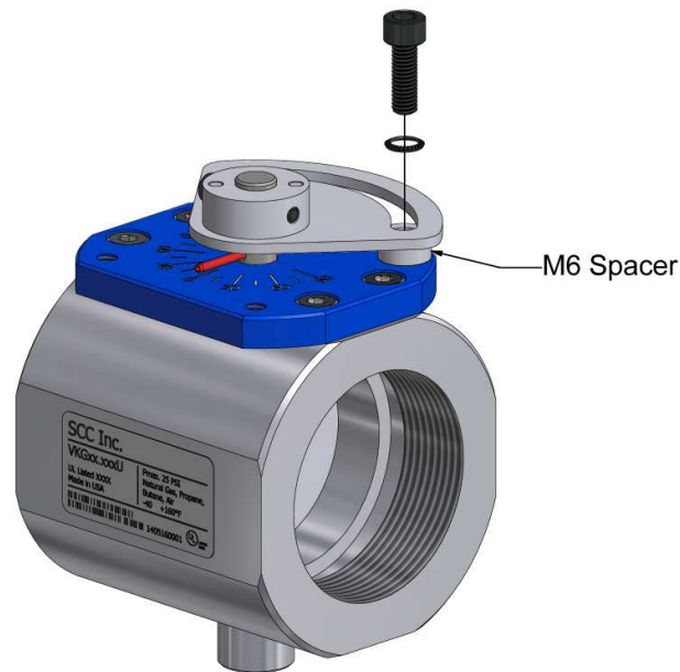
Figure 3: Completed Installation of AGA92.2 Manual Kit
