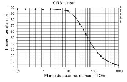
A flame detector resistance of RF <500  $\Omega$  is identified as a short-circuit and leads to safety shutdown in operation, like in the case of loss of flame.
